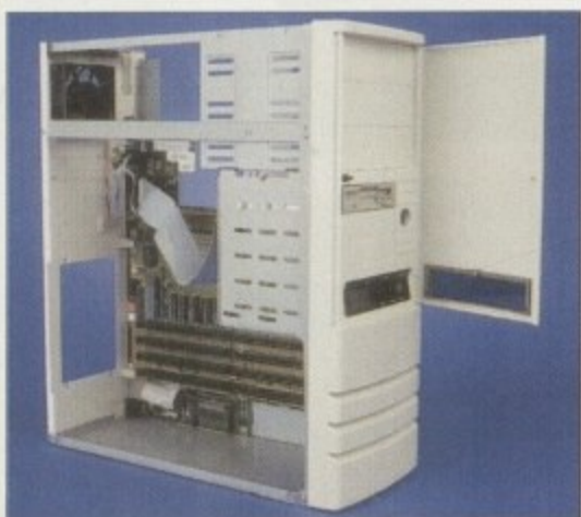
Things are looking cool already. As you can see, the floppy disk in the drive cage is poking out through the drive bay slot nice and flush
